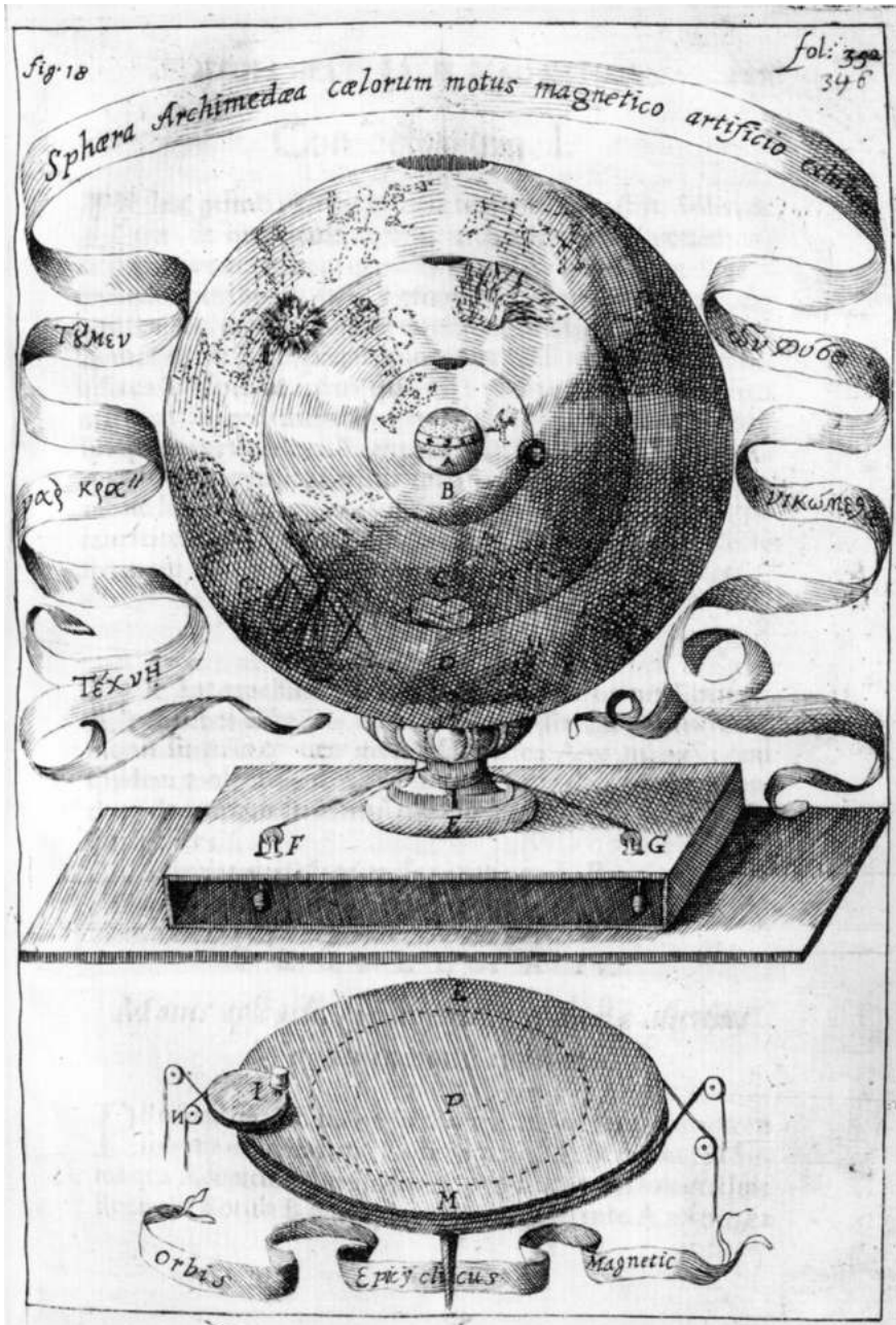
Figure 12. An Illustration showing some of the behind-the-scene functionality of a particular “magnetic epicyclic disk.” Each sphere was filled with clear oil and water, which would not mix, allowing for objects therein to appear suspended, when they were actually floating. Magnets, thin silk threads, and a hidden pulley system rotated the balls, suggesting certain arrangements of planets and constellations, which was not entirely accurate. The combination of orientations would also be taken as a horoscope—with the same fun attitude that one has when interacting with a magic 8 ball, a Ouija board, or a mood ring. Here the objects “seem to move of their own accord but are in fact controlled by concealed magnets.”
